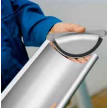
Flat End Cap with Rubber Seal These end caps are self-sealing with an EPDM tube. They are fully reversible, i.e. same unit fits on both left and right end of a gutter. And they are easily mounted with just a single, firm knock.
