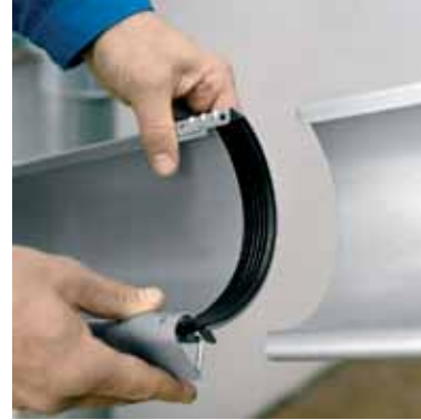
Gutter Connector with Rubber Seal The gutter connector is easy to fit and allows the joining of two sections of gutter without the need to use a silicon calking adhesive. Simply leave a 1/8" -1/4" gap between the two sections of gutter to be joined and connect using our easy to install gutter connector. The result is a very firm and durable connection. The EDPM seal is long lasting and guaranteed leak proof.
